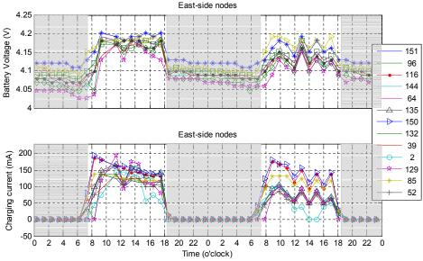
Figure 11: Monitored battery voltage and charging current.
