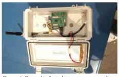
Figure 4: Example of wireless smart sensor nodes deployed on the Jindo Bridge.
