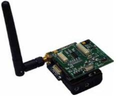
Figure 2: Imote2/ISM400 wireless smart sensor node.
